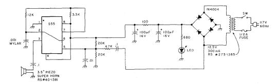
Fig. 1. Ultrasonic bug-chaser schematic.
